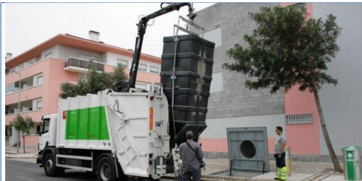
Figure 5: underground container during collection (source: Cascais Municipality website)
