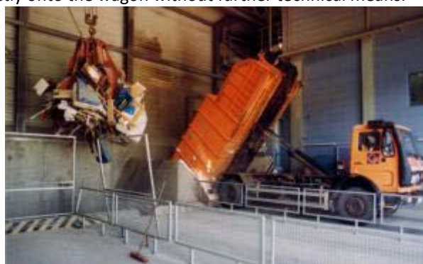
Figure 4: Waste transfer station with a ramp for the unloading of the collection vehicle and an excavator for reloading the waste (Picture source: Intecus GmbH)
