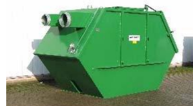
Figure 5: Skip container version for the separation of wooden chips
