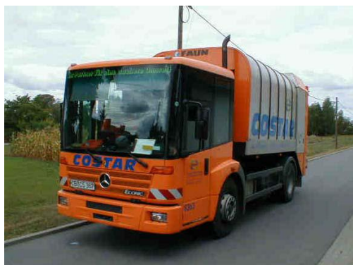
Pic. e: Vehicle with screw-type rotating drum and low-entry cabin 'Econic'
