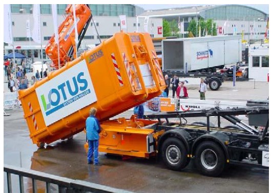
Pic. f: Special version of rear-end loaded vehicle with swap body (with feed hopper and lifting device turned down for container unload)
