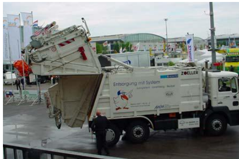
Pic. c: double body vehicle for the parallel collection of two of source-separated waste fractions. (with one feed hopper opened for discharge)
