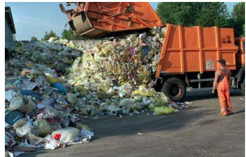
Pic. d: Emptying of a rear-end loaded vehicle with the help of the ejection plate
