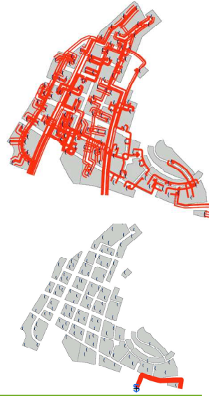
Picture 3. Comparison of an assessment of the collection route intensity of conventional waste handling and underground waste transportation in a residential area to be built in Stockholm
