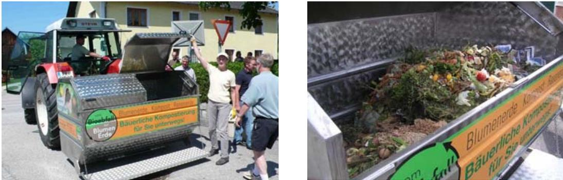
Figure 2. Collection container attached to the back of a tractor
