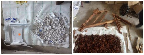
Figure 23: plastic (left) and wood (right), before and after fragmentation
